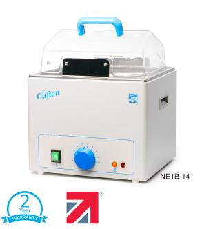
Designed for applications that require continuous boiling. This bath also has the flexibility where the control can be regulated from a gentle simmer to a vigorous boil.
